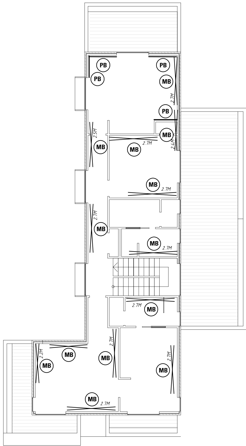
FIRST FLOOR BRACING PLAN SCALE 1:100
