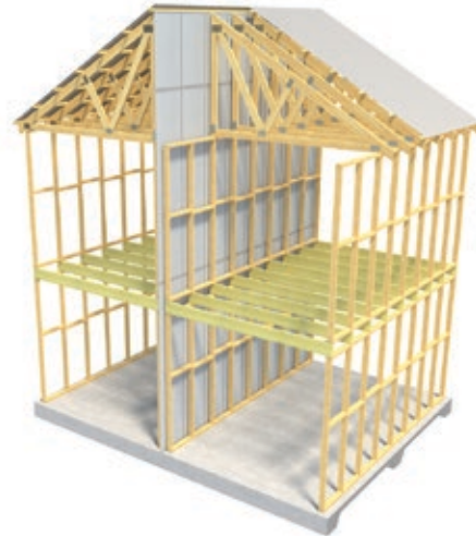
Figure 2: Partiwall Design Concept
